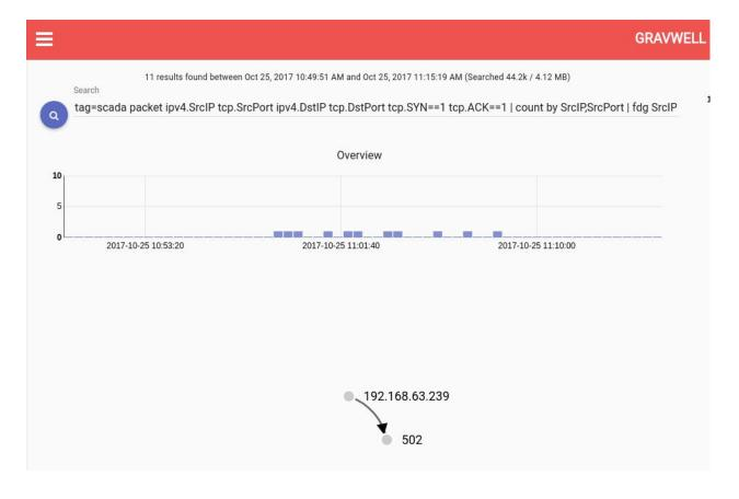
```tag=scada packet ipv4.SrcIP tcp.SrcPort ipv4.DstIP tcp.DstPort tcp.SYN==1
